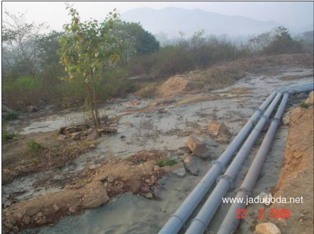
Figure 9a. According to the SME Surface Mining Handbook , “For quite some time, the mining industry has been dealing with the problems and consequences caused by pipeline failures. Failures often result in environmental damage that may affect people that live near pipelines (e.g., in the case of water or land contamination, or as a direct effect of flooding populated areas) ... In addition, there are the human and environmental impacts. A failure in a slurry pipeline may involve fatal events and environmental contamination, which can affect the livelihood of local habitants” (Ihle and Valencia, 2023). On February 21, 2008, a new tailings pipeline burst near Jaduguda in the state of Jharkhand, India, causing a spill of uranium mill tailings that reached nearby homes. Photo from WISE Uranium Project (2008).
