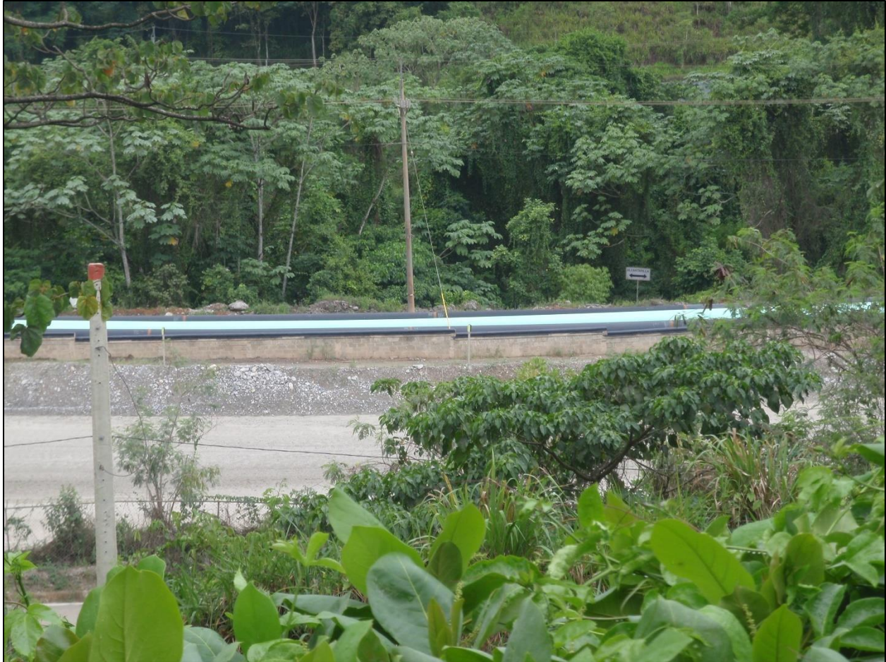
Figure 8. At the Barrick Pueblo Viejo gold mine in the Dominican Republic, tailings are transported by pipeline about 3.5 kilometers from the ore processing plant to the El Llagal tailings storage facility. Photo taken by the author on July 13, 2023.
